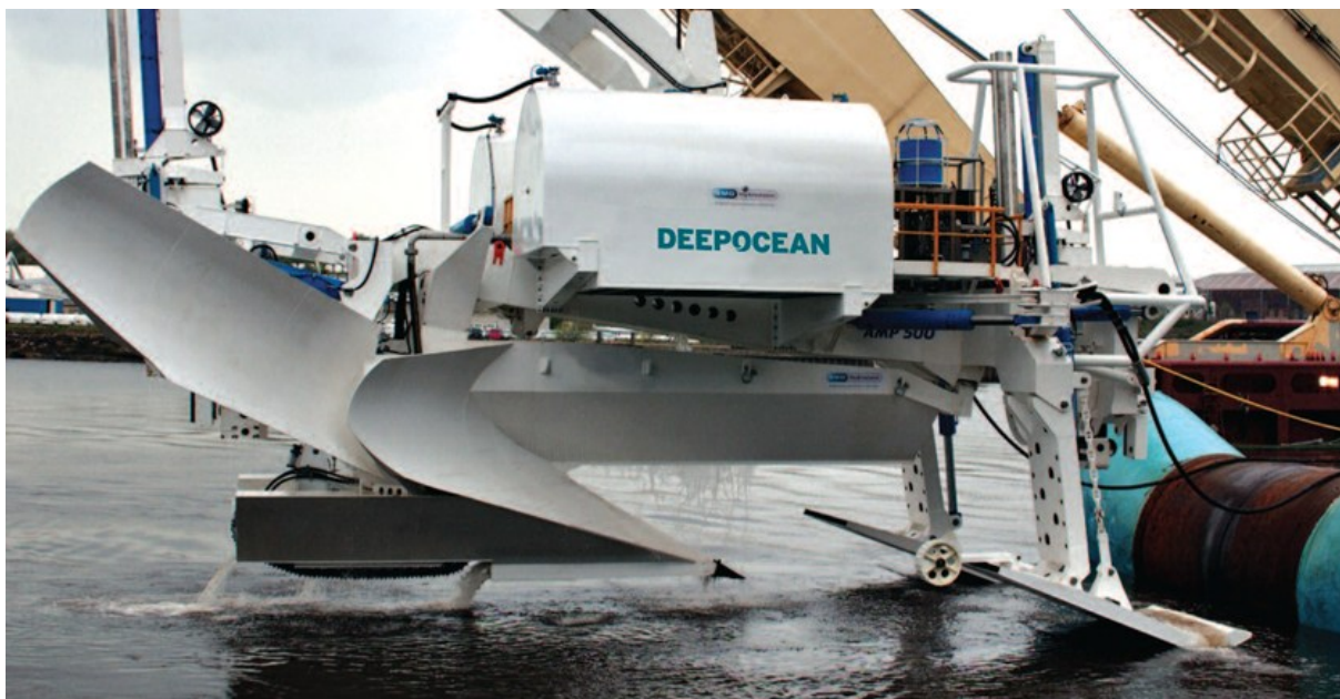
Figure 3.15 AMP500 advanced multi-pass plough. Source: https://www.subsea-rov.com/services-assets/trenchers-ploughs/item/74-amp500
