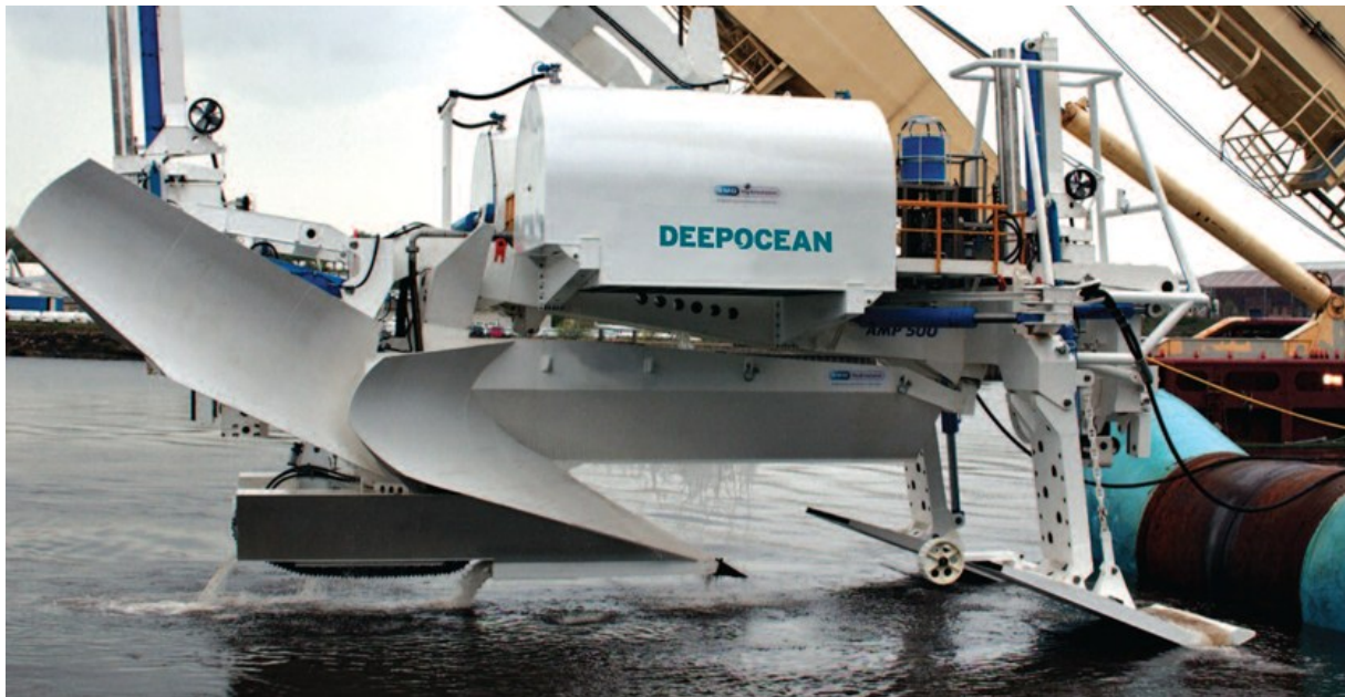
Figur 3.15. Avancerad multipass-plog AMP500. Källa: https://www.subsea-rov.com/services-assets/trenchers-ploughs/item/74-amp500
