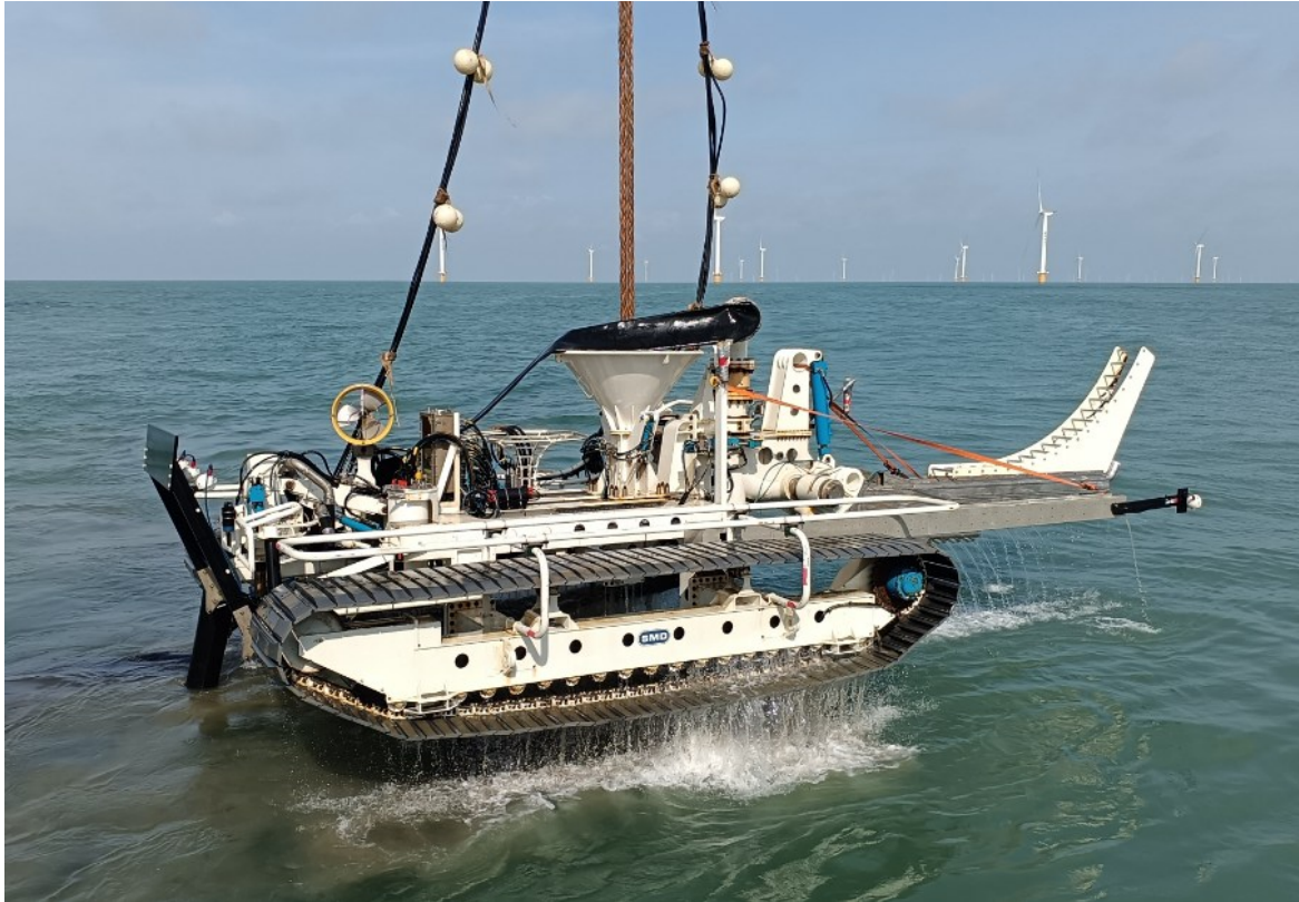
Abbildung 3.13 Bagger für Flachwassergraben (Shallow Water Trencher)(Quelle: https://www.smd.co.uk/blog/may-2023-smds-shallow-water-trencher-the-story-so-far/ )
